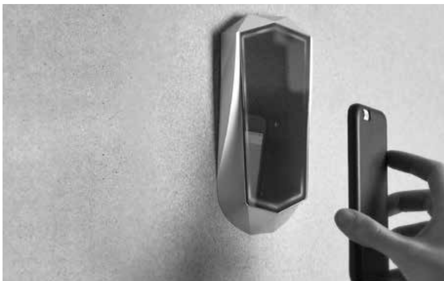
The LightPass is called up on the smartphone and scanned using a reader.
